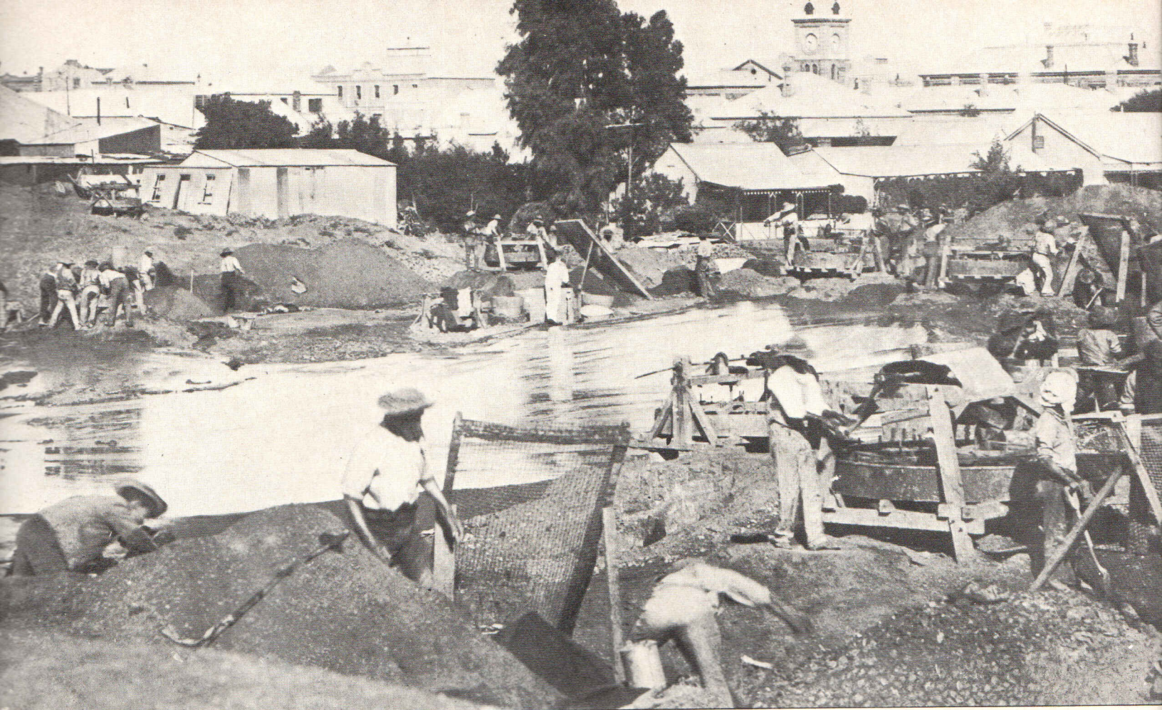
After sieving the diamond-bearing soil, many diggers washed the material in hand-rotated drums to reveal the elusive stones.
